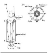
The drawing (a) represents a general overview of the Ilizarov technique. (b) Represents a cross section.
